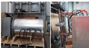
Current withstand test
